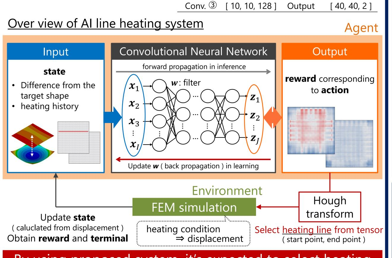
By using proposed system, it's expected to select heating line that can obtain a closest shape to the target shape
