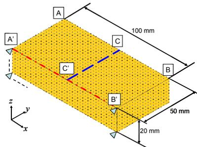
Fig.3 Computational model of bead-on-plate and analysis condition
