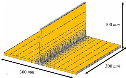
Fig.9 Numerical model of nodal point distributions of T welded joint and that of xy cross-section
