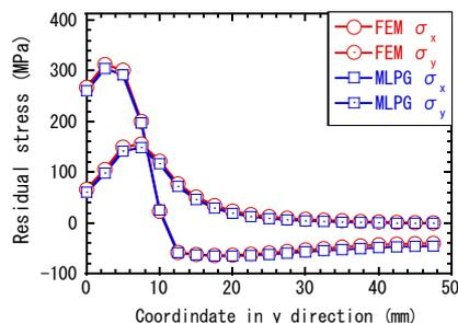
Fig.4 Comparison of residual stress of FEM with MLPG on top surface of transverse cross section
