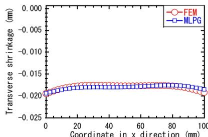
Fig.6 Comparison of transverse shrinkage between FEM and MLPG on top surface of A-A' to B-B'
