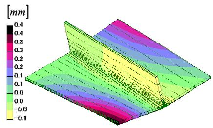
Fig.11 Distribution of displacement in z direction
