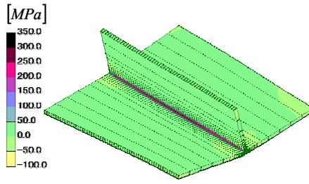
Fig.10 Distribution of residual stress in x direction
