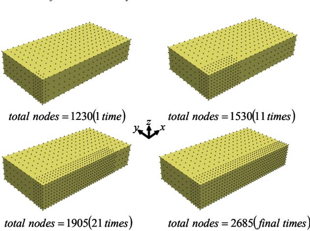
Fig.12 Computational model after adding nodes
