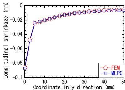
Fig.5 Comparison of longitudinal shrinkage between FEM and MLPG on top surface of A-B to A'-B'
