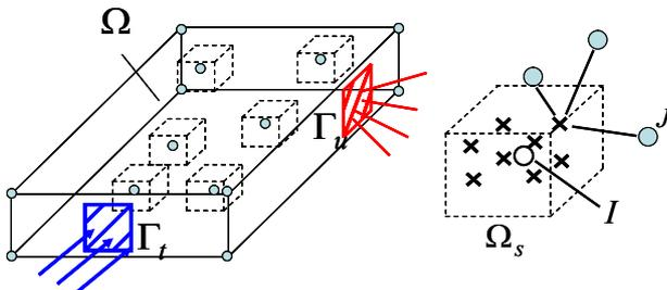
Fig.2 Schematic illustration of local domain of MLPG
