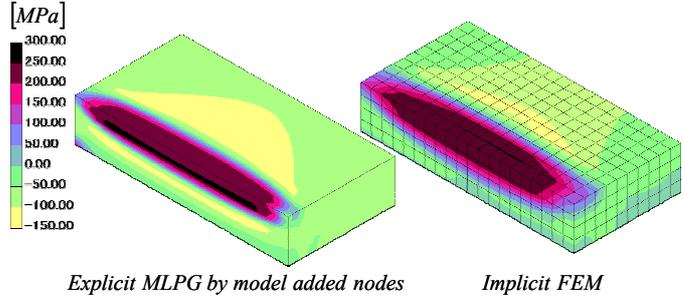
Fig.13 Distributions of residual stress in x direction
