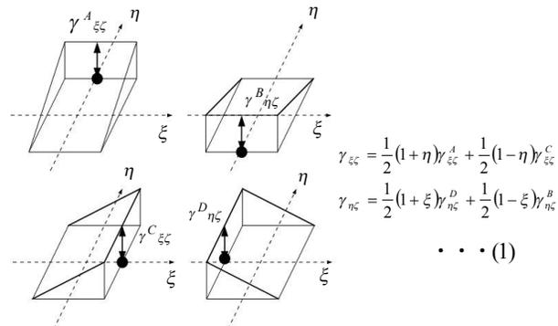
Fig. 1 Sampling points of transverse shear strain of MITC4
