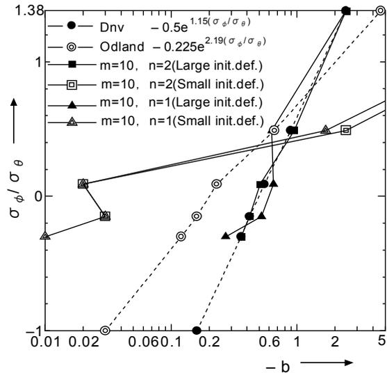
Fig. 7 b-factor for the spherical shell segments
