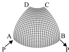
Fig. 4 Hemispherical shell with 18° hole
