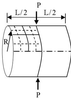
Fig. 3. Pinched cylinder with rigid end diaphragms
