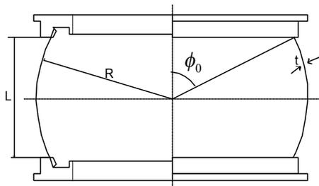
Fig. 6 Toroidal Shell Segment model
