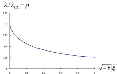
Fig. 5 Effect of initial deflection and b-factor on knockdown factor
