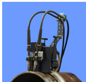
Fig. 2 Photo of tandem welding head.
